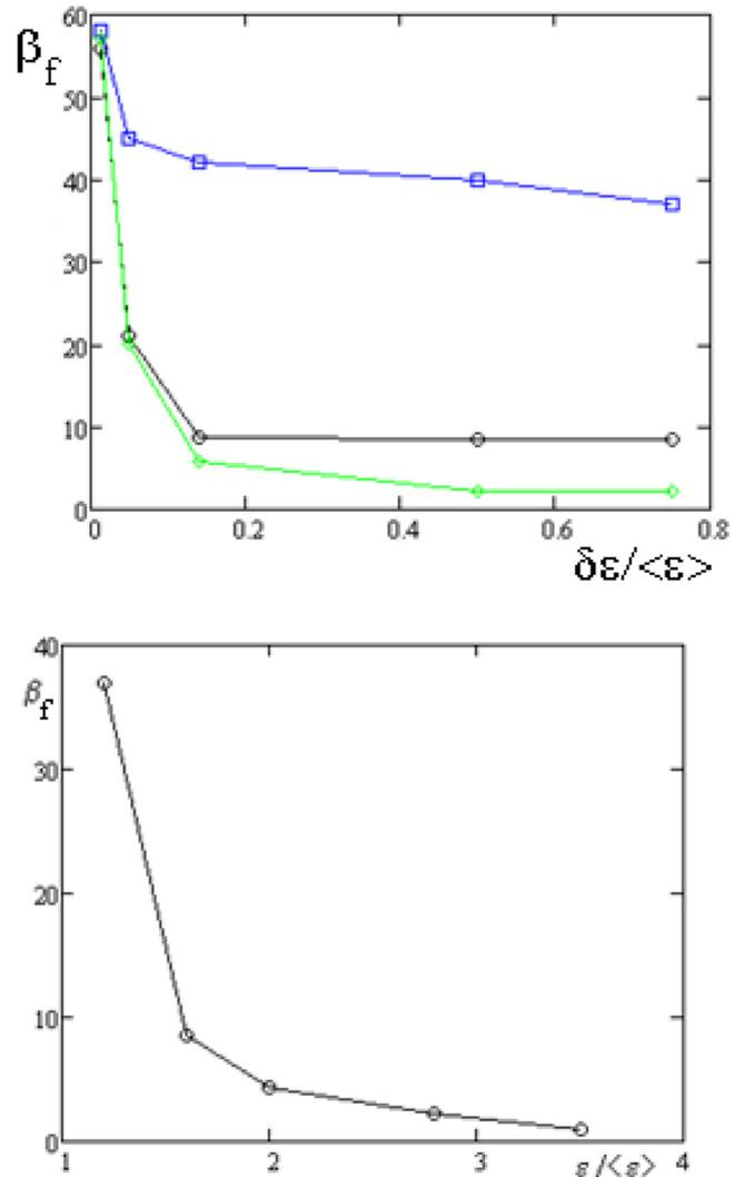
FIG. 7. (a) Optimal value of parameter  $\beta_f$  as function of  $\delta\varepsilon/\langle\varepsilon\rangle$  and  $T_{e2}/\langle\varepsilon\rangle = 0.2$  (blue line), 0.6 (black line), and 1.8 (green line). (b) Dependence of optimal value of  $\beta_f$  on the normalized energy enhancement.
