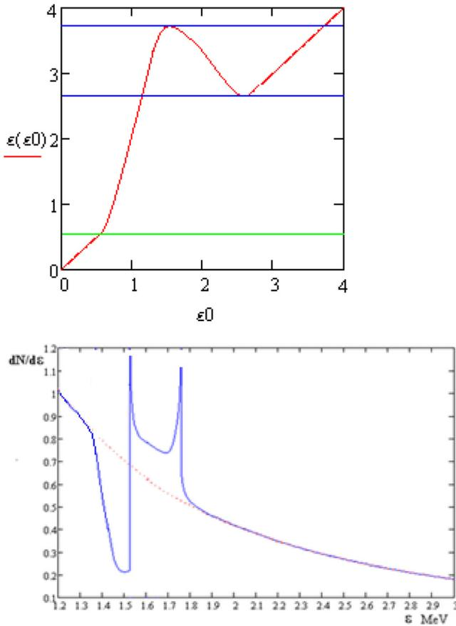
FIG. 4. (a) Function  $\varepsilon(\varepsilon_0)$  for the accelerating triangular field; (b) distribution function of protons with smooth distribution function (red lines) after transition through the accelerating field. Calculation parameters are:  $l_1 = 5 \mu\text{m}$ ,  $\varepsilon_{12} = 1.5 \text{ MeV}$ ,  $T_{e2} = 0.3 \text{ MeV}$ ,  $\tau_f = 200 \text{ fs}$ , and  $\nu = 10^{-3}$ .
