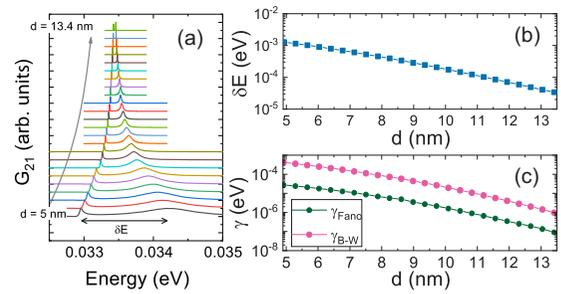
FIG. 4. (a) Conductance spectra around the first resonance peaks as functions of Dirac fermion energy for various edge-dot distances from  $d = 5$  to  $13.4$  nm with an increment  $0.37$  nm. (b) The energy splitting  $\delta E$  as a function of  $d$  from the fitted data. (c) Coupling strengths of Fano and Breit-Wigner resonances,  $\gamma_{\text{Fano}}$  and  $\gamma_{\text{BW}}$ , from the numerical fitting as functions of  $d$ .
