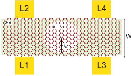
FIG. 1. Schematic diagram of the system considered in this work. The external magnetic field is expelled out in the circular area characterized by radius  $r_0$ . There are four leads labeled as L1, L2, L3, and L4 for scattering matrix calculations from a lead to another lead.
