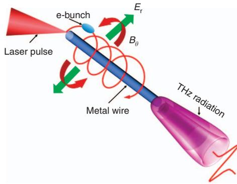
**Figure 1** A schematic view of the laser-driven-wire-guided undulator (LWGU) developed at SIOM. A femtosecond laser pulse irradiating a metal wire emits an energetic electron bunch. Concurrently, a highly positive transient current excites an outward-pointing radial electric field ( $E_r$ ) and azimuthal magnetic field ( $B_\theta$ ) along the wire. The laser-generated fast electrons undergo helical betatron motion due to strong Lorentz forces and emit amplified THz radiation.
