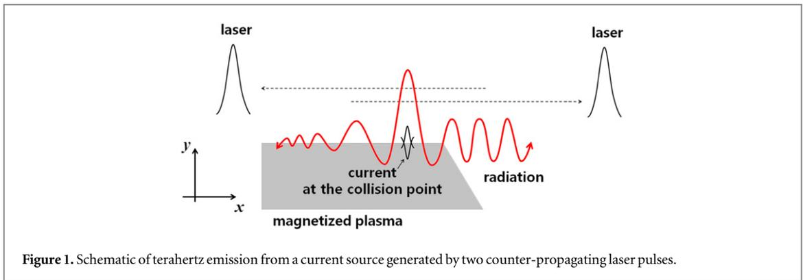
Figure 1. Schematic of terahertz emission from a current source generated by two counter-propagating laser pulses.
