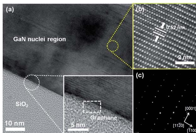
**Fig. 4** (a) Low-magnification cross-sectional TEM image of GaN nuclei region on graphene. The number of graphene layers is shown in the inset image. (b) The corresponding high-resolution TEM image. (c) Electron diffraction pattern of GaN crystal grown on Gr/SiO<sub>2</sub>/Si.
