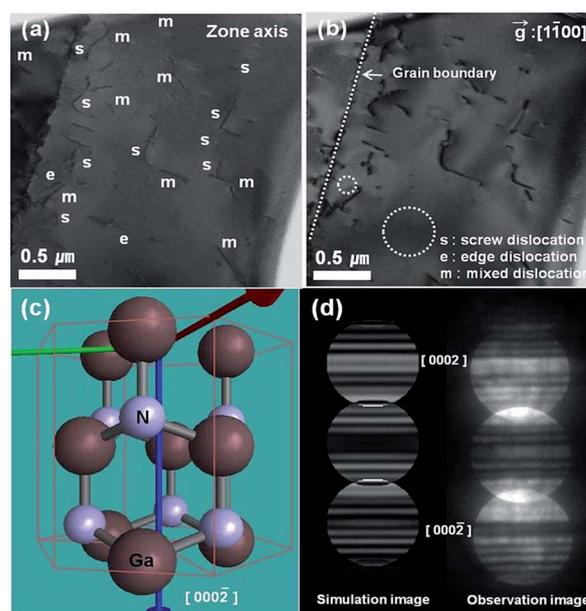
**Fig. 5** Cross-sectional two-beam bright-field TEM images of GaN crystal on graphene: (a) zone axis and (b)  $g = [1100]$  image showing screw and mixed dislocations. (c) Convergent beam electron diffraction (CBED) simulation structure of stacking-grown GaN on Gr/SiO<sub>2</sub>/Si and (d) simulated and observed CBED patterns for 160 nm thickness.
