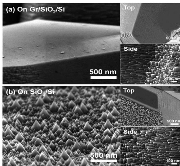
Fig. 6 FESEM images of GaN grown on (a) Gr/SiO<sub>2</sub>/Si and (b) SiO<sub>2</sub>/Si after etching for 20 min in 0.5 mol KOH. The right images show top and side views of GaN after etching.
