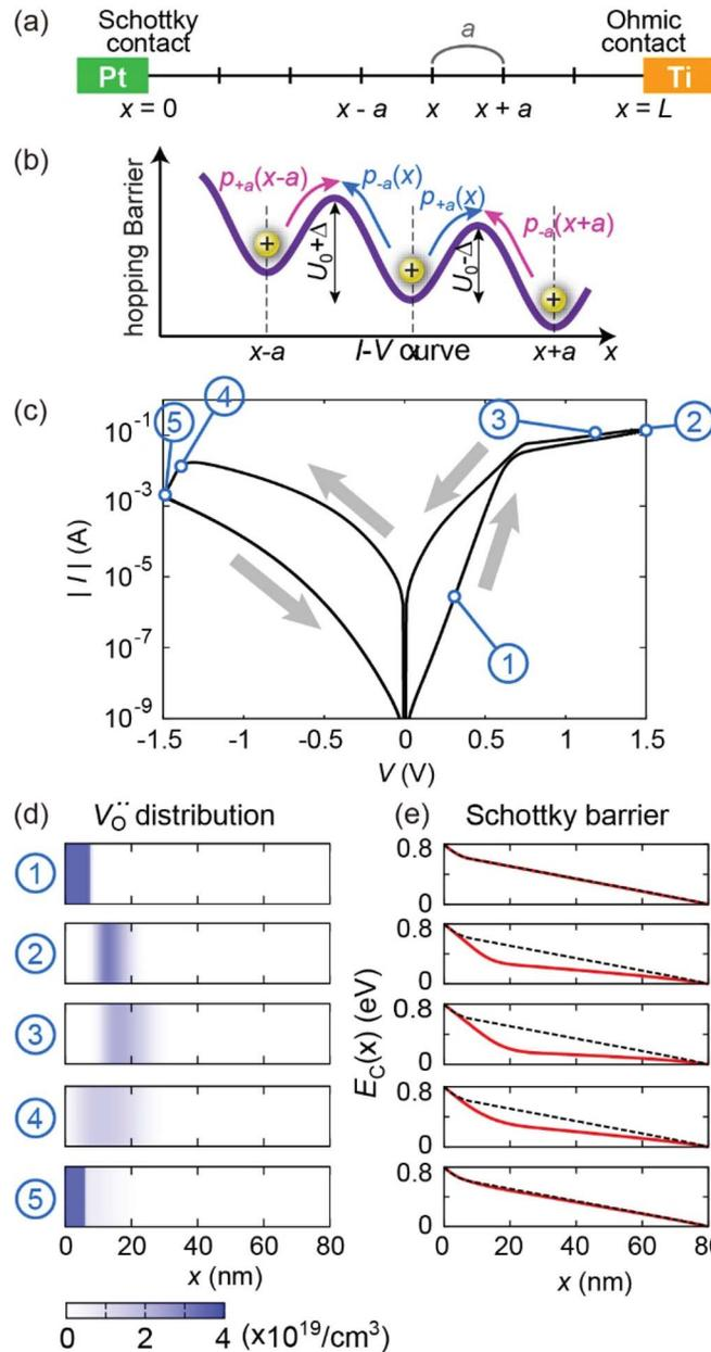
FIG. 3. Results of SMD model simulations. (a) Simple one-dimensional lattice used in the simulation. (b) Hopping probabilities for  $V_o''$  to overcome a hopping barrier. (c) Simulated f8  $I$ - $V$  curve of a Pt/Nb:SrTiO<sub>3</sub> cell. (d) Calculated  $V_o''$  distribution across the sample. The numbers indicate each resistance state of the simulated f8  $I$ - $V$  curve. (e) Associated Schottky barrier changes coming from  $V_o''$  redistribution.
