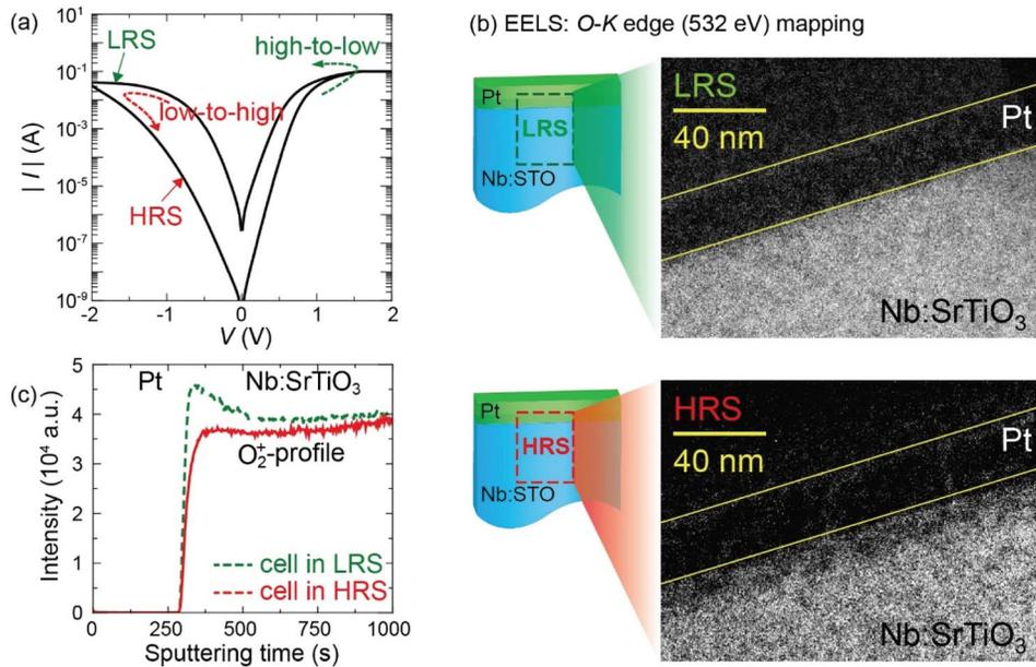
FIG. 2. (a) Experimental  $I$ - $V$  curves for a BRS Pt/Nb:SrTiO<sub>3</sub> cell. (b) EELS O-K (O 1s  $\rightarrow$  2p, 532 eV) edge mapping images of the LRS (upper) and the HRS (lower). (c) Collected SIMS signals for ejected secondary O<sup>2+</sup> ions across the interface for a cell in the LRS (green dashed line) and the HRS (red solid line).
