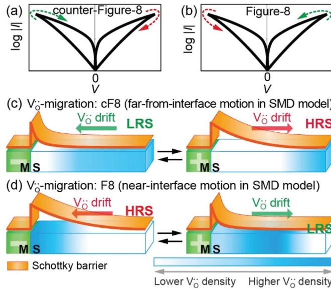
FIG. 1. SMD model of BRS phenomena. The mobile dopants are  $V_o''$ . (a) cf8 and (b) f8  $I$ - $V$  curves. (c) SMD model for cf8-type. The  $V_o''$  move far from the interface. (d) SMD model for f8-type. The  $V_o''$  move near the interface.
